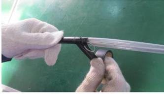
1. Remove the sheath of the optic cable. Spare 1.1-1.6m bare fibers and keep 30-50mm length of the strength member wire. Bend the wire  $> 90^\circ$ . Put the bare fibers through the transparent tube. Use PVC tape to wrap the joint places of the cable and the transparent tubes.
